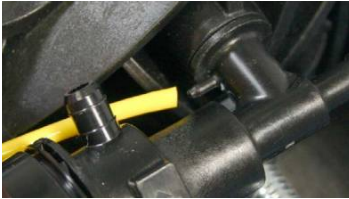
Figure 8-11: PRESSURE LINE REMOVAL
